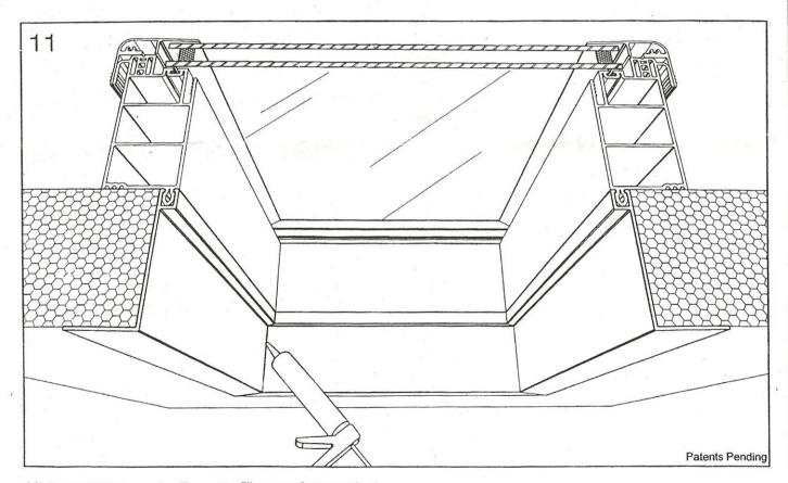
11) If necessary, apply silicone to fill gaps along vertical corners.
