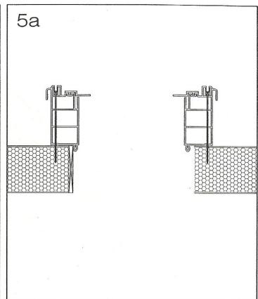
5) Fasten skylight to roof panel with 3/16" socket drive head, #10 5 1/4" screws. 5a) Remove shims
