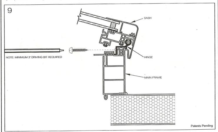
9) Fasten sash to main frame in pre-drilled holes located on hinge using fasteners supplied.
