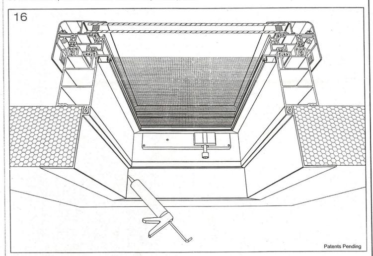
16) If necessary, apply silicone to fill gaps along vertical corners.
