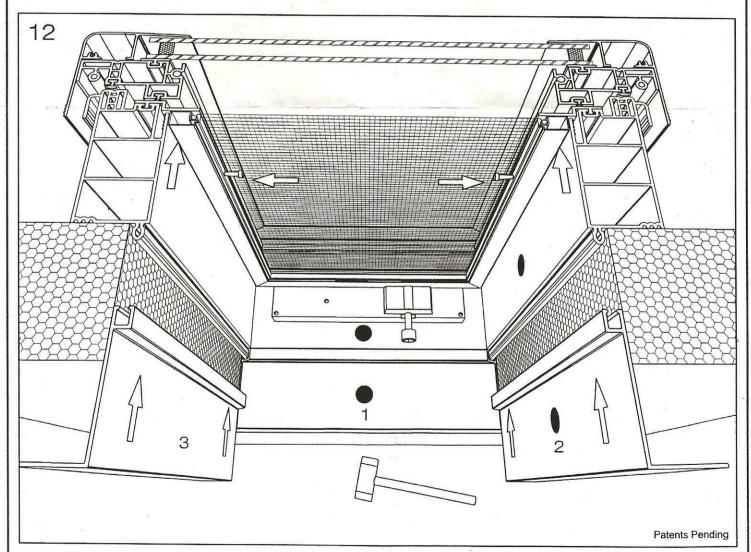
12) Your snap-on covers are cut to exact dimensions, individually fitted with sides of skylight frame and are referenced with matching color dots for proper placement and installation.
