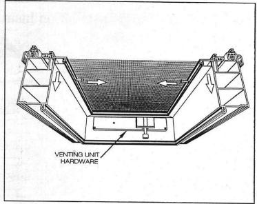
Handle With Caution! Venting unit sash is not fastened to main frame on header. Open venting sash to maximum height, remove pin from hardware, separate sash from main frame and remove insect screen.
