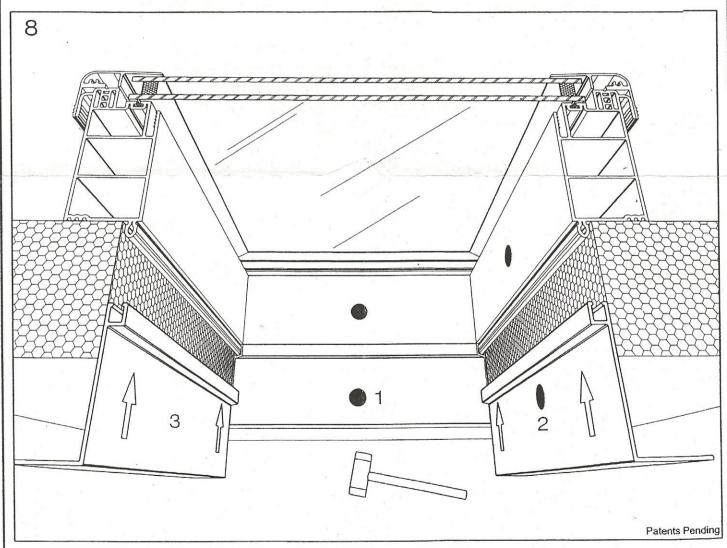
8) Your snap-on covers are cut to exact dimensions, individually fitted with sides of skylight frame and are referenced with matching color dots for proper placement and installation.
