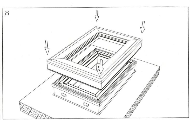
8) Before installing sash, make sure hardware chain link is in maximum opening position. Now you're ready to install sash to main frame. Hinging system is designed and cut to interior width of main frame. Lift bottom of sash to an open position and hinge will drop and self position sash to main frame for proper alignment. (Refer to step 9).
