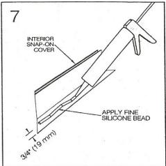
7) Apply a fine silicone bead to bottom legs of interior snap-on covers to avoid bowing and to assure proper alignment and adhesion to interior of roof panel.
